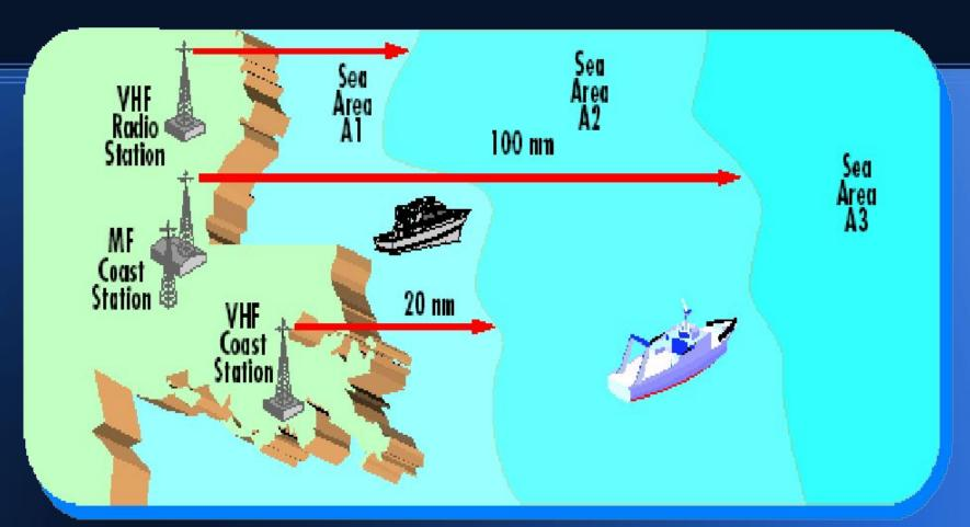
Sea area A1 -The area within the radiotelephone coverage of at least one very high frequency (VHF) coast station in which continuous DSC alerting is available
