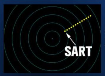
In passive mode batteries last 96 hours – can actively respond to radar signal for 8 hours
